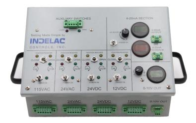
THIS TEST BOX WAS DESIGNED TO TEST THE <u>MAJORITY</u> OF <u>INDELAC</u> ACTUATORS, WITH AND WITHOUT MODULATING BOARDS AND TRANSMITTERS. THIS IS MAINLY USED FOR PRODUCTION BENCH CALIBRATION AND TESTING OF <u>INDELAC</u> ACTUATORS AS A STAND ALONE OR WITH A VALVE ATTACHED.
