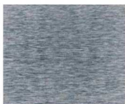
Surface finish: fine-machined, and grinded, Ra 0.2 \mu\text{m}
