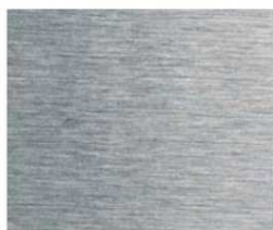
Surface finish: machined, Ra 0.8 \mu\text{m}
