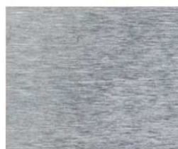
Surface finish: fine-machined, and grinded, Ra 0.4 \mu\text{m}
