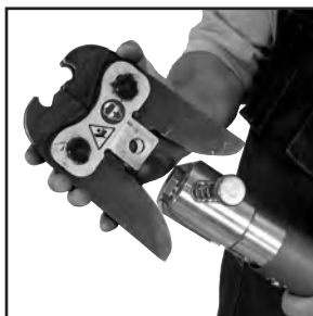
Figure 7: Placement of adapter jaw into the tool
