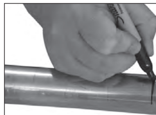
Figure 3 — Marking for Insertion Depth
