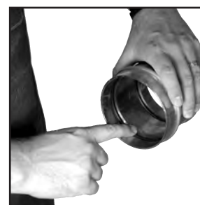
Figure 5: Check for EPDM seal
