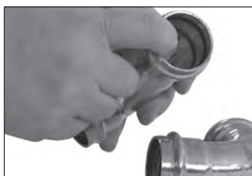
Figure 2 — Check for EPDM Seal
