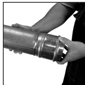
Figure 9: Inspection of final crimp
