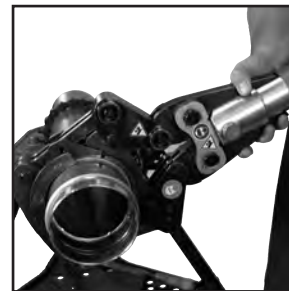
Figure 8: Placement of adapter jaw into pressing chain
