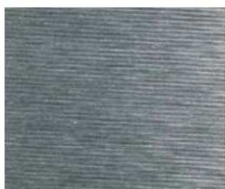
Surface finish: machined, Ra 1.2 \mu\text{m}
