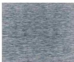
Surface finish: fine-machined, and grinded, Ra 0.2 \mu\text{m}
