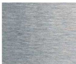
Surface finish: machined, Ra 0.8 \mu\text{m}
